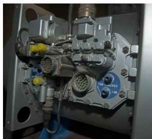
Figure 4. Fuel cell utilised in service module for command electrical power on the Gemini missions.
